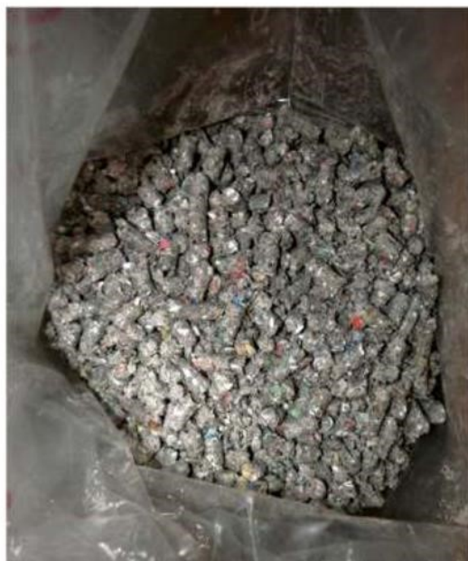
Fig. 2 – «Type 1» with 50% HDPE-PP sample
